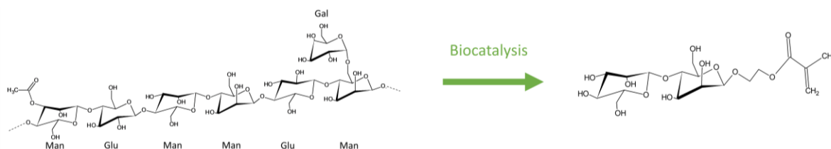
Figure 1. Schematic representation of target glycosyl substrate, AcGGM, and product, \beta -mannobiosyloxyethyl methacrylate from TrMan5A biocatalysis.
